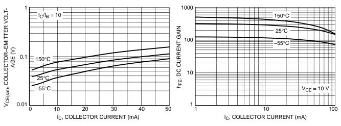
Figure 7. V<sub>CE(sat)</sub> vs. I<sub>C</sub>
