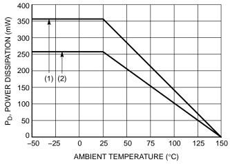
Figure 1. Derating Curve
