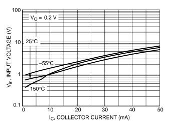
Figure 11. Input Voltage vs. Output Current
