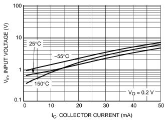
Figure 6. Input Voltage vs. Output Current
