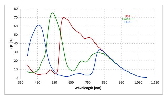
Figure 12. RGB Quantum Efficiency Curve
