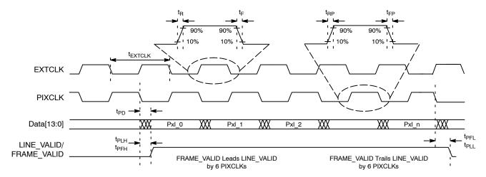
Figure 14. I/O Timing Diagram
