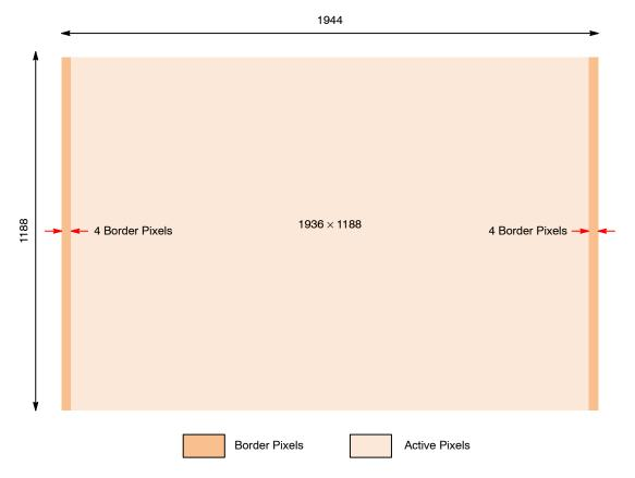
Figure 5. Pixel Array Description
