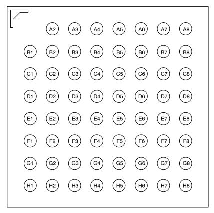
Figure 4. 63-ball iBGA Package (Top View)
