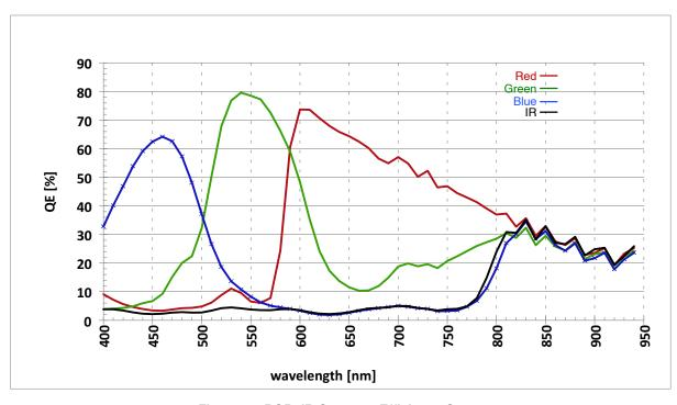
Figure 13. RGB-IR Quantum Efficiency Curve
