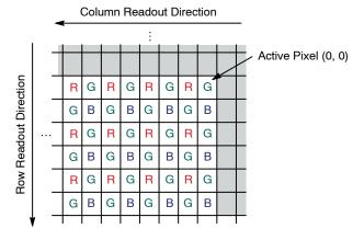
Figure 6. Pixel Color Pattern Detail (Top Right Corner)
