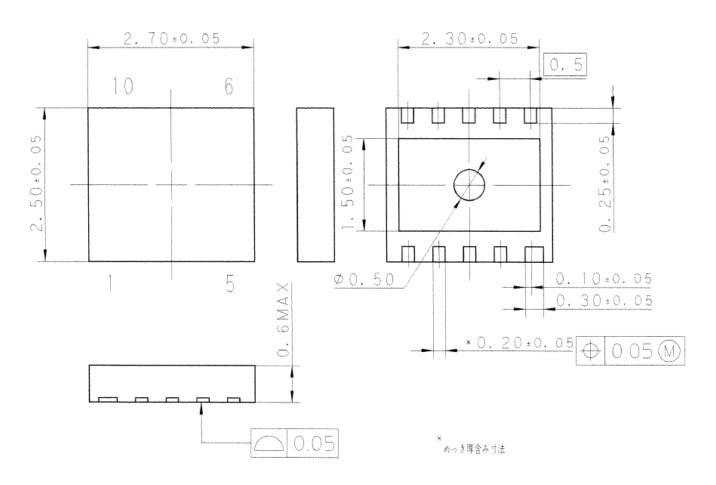
Dimension including the plating thickness
