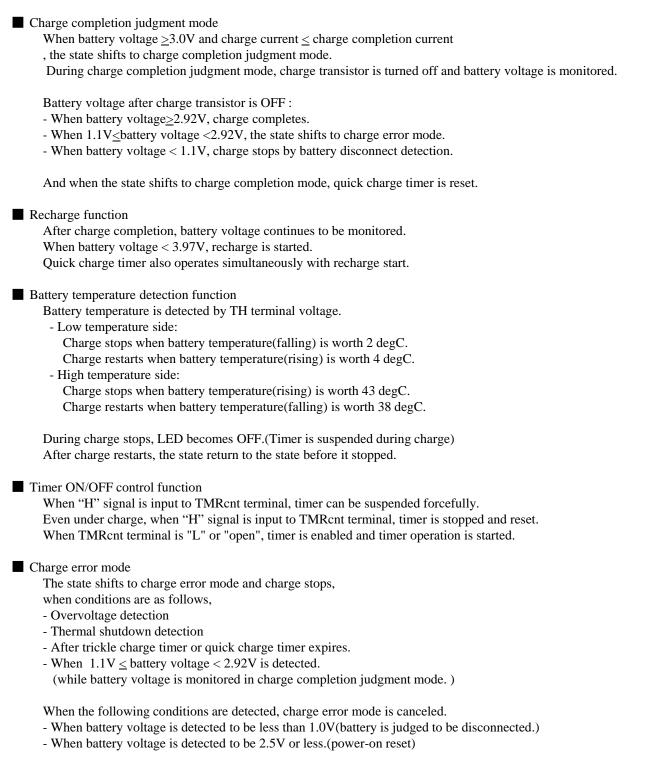
While charge error mode, the battery discharge current is 10uA.
