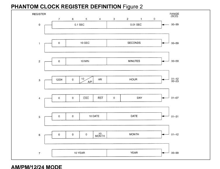
Bit 7 of the hours register is defined as the 12-hour or 24-hour mode-select bit. When high, the 12-hour mode is selected. In the 12-hour mode, bit 5 is the AM/PM bit with logic high being PM. In the 24-hour mode, bit 5 is the second 10-hour bit (20–23 hours).
