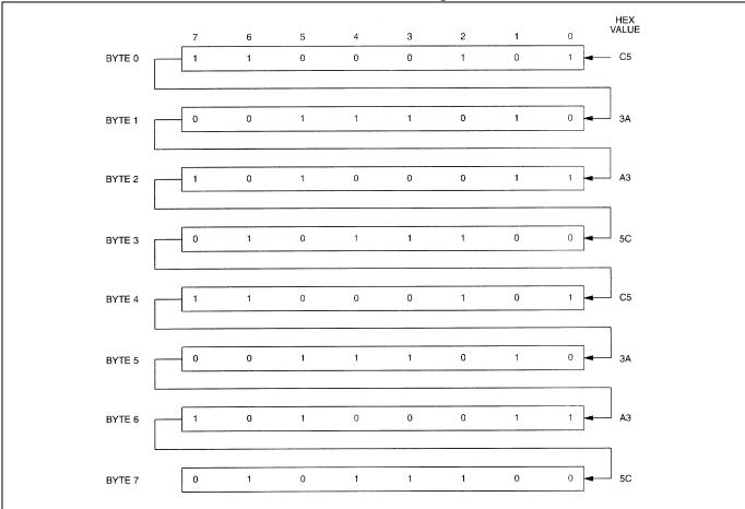
**NOTE:** THE PATTERN RECOGNITION IN HEX IS C5, 3A, A3, 5C, C5, 3A, A3, 5C. THE ODDS OF THIS PATTERN BEING ACCIDENTALLY DUPLICATED AND CAUSING INADVERTENT ENTRY TO THE PHANTOM CLOCK IS LESS THAN 1 IN 1019. THIS PATTERN IS SENT TO THE PHANTOM CLOCK LSB TO MSB.
