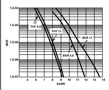
FIGURE 16. BER vs EB/N0 PERFORMANCE FOR MBOK MODES
