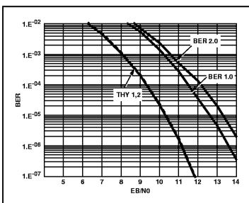
FIGURE 15. BER vs EB/N0 PERFORMANCE FOR PSK MODES
