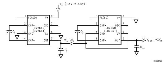
FIGURE 5. Increasing Output Voltage by Cascading Devices
