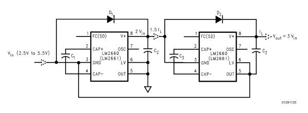
FIGURE 7. Generating +3V<sub>in</sub> from +V<sub>in</sub>
