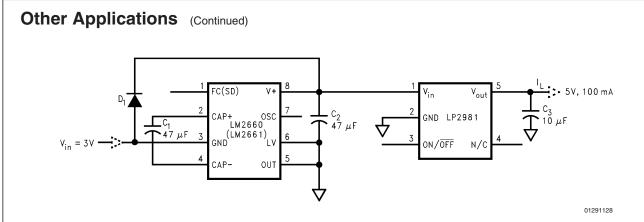
FIGURE 9. Generating +5V from +3V Input Voltage
