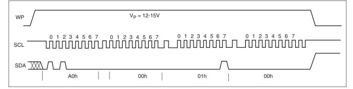
Figure 1. Set V<sub>TRIP</sub> Level Sequence (V<sub>CC</sub> = desired V<sub>TRIP</sub> values WEL bit set)
