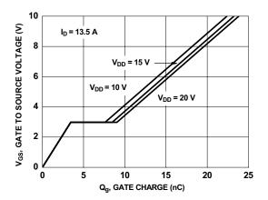
Figure 7. Gate Charge Characteristics
