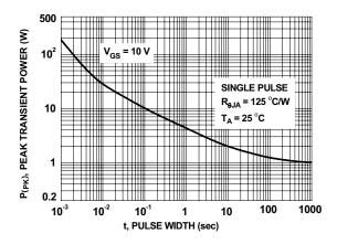
Figure 12. Single Pulse Maximum Power Dissipation
