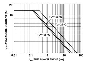
Figure 9. Unclamped Inductive Switching Capability
