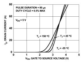
Figure 5. Transfer Characteristics
