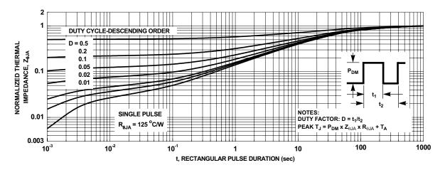
Figure 13. Junction-to-Ambient Transient Thermal Response Curve
