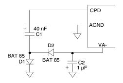
Figure 5. Generating VA- with a Charge Pump
