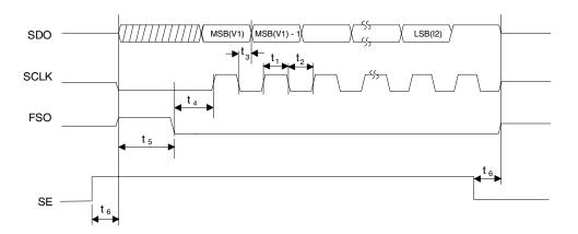
Figure 1. Serial Port Timing
