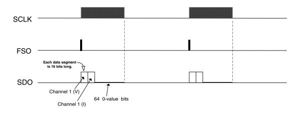
Figure 3. Serial Port Data Transfer
