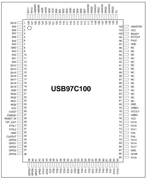
FIGURE 1 - PIN CONFIGURATION
