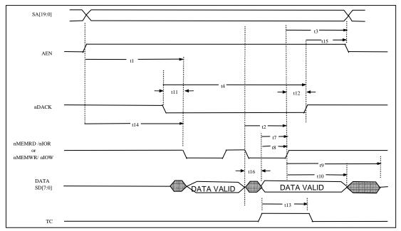
FIGURE 14 - DMA TIMING (BURST TRANSFER MODE)
