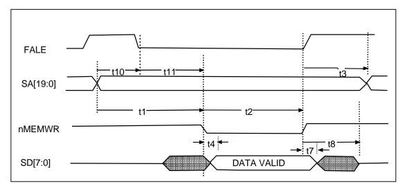
FIGURE 17 - 8051 FLASH MEMORY WRITE TIMING
