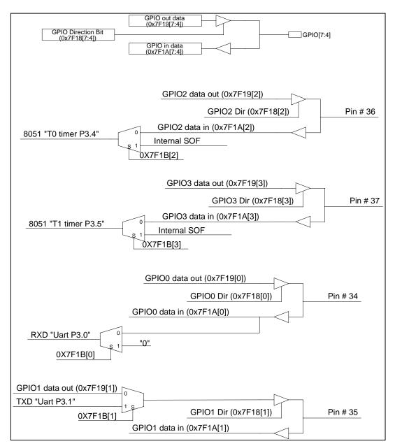
FIGURE 3 - GPIO MUXING BLOCK DIAGRAM
