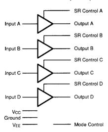
Logic for Am26LS30 with Mode Control LOW (RS-422)
