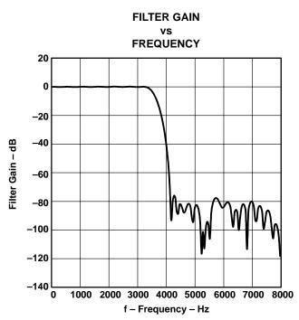
Figure 5–18. DAC FIR Frequency Response (OSR = 128)
