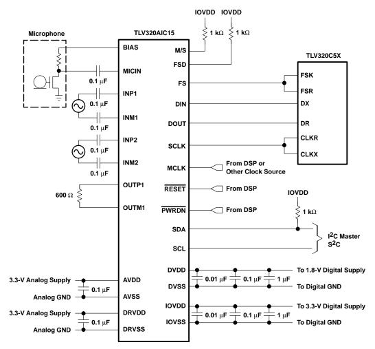
Figure 5–19. Single-Ended Microphone Input (Internal Common Mode)
