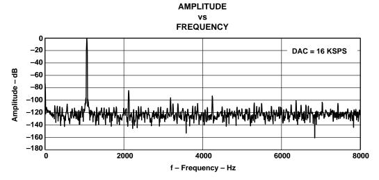
Figure 5-7. FFT—DAC Channel (0 dB Input)
