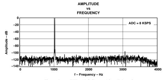
Figure 5-10. FFT—ADC Channel (-1 dB Input)
