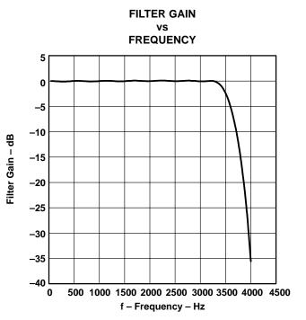
Figure 5-11. ADC FIR Frequency Response
