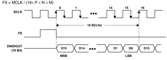
Figure 3-5. Timing Diagram of FS
