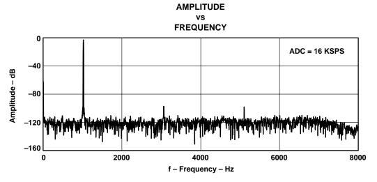
Figure 5-5. FFT—ADC Channel (-3 dB Input)
