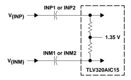
Figure 3-2. INP and INM Internal Self-Biased Circuit
