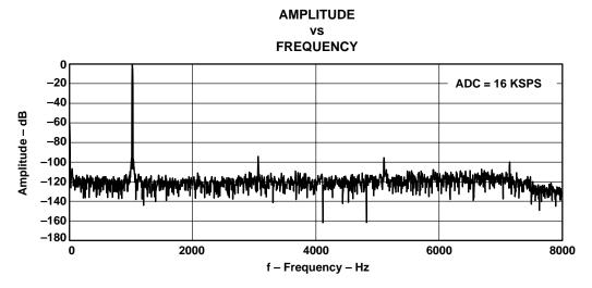
Figure 5-4. FFT—ADC Channel (-1 dB Input)
