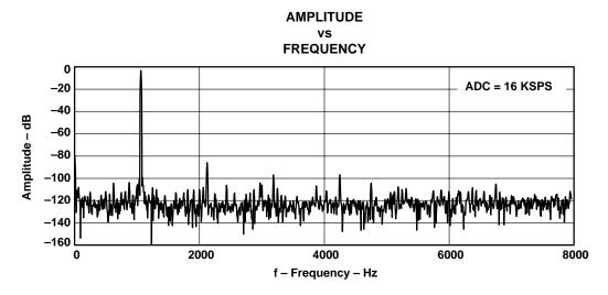
Figure 5-6. FFT—DAC Channel (-3 dB Input)
