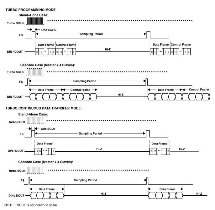
Figure 3-17. Timing Diagram for Turbo Operation
