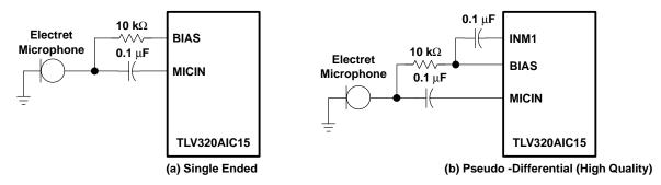
Figure 3-1. Microphone Interface
