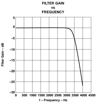
Figure 5-12. ADC IIR Frequency Response
