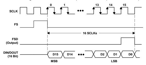
Figure 3-6. Timing Diagram for FSD Output
