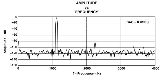
Figure 5-8. FFT—DAC Channel (-3 dB Input)
