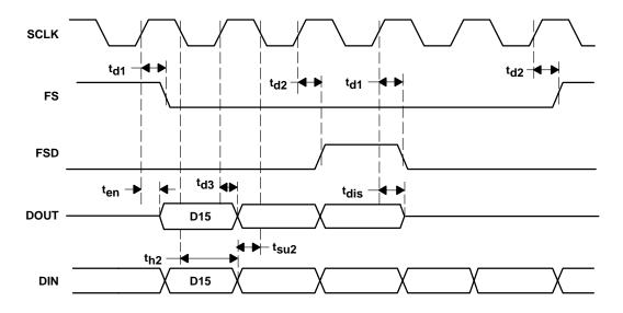
Figure 5–2. Serial Communication Timing
