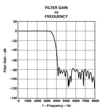
Figure 5–17. DAC FIR Frequency Response (OSR = 256)
