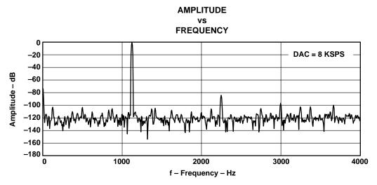
Figure 5-9. FFT-DAC Channel (0 dB Input)
