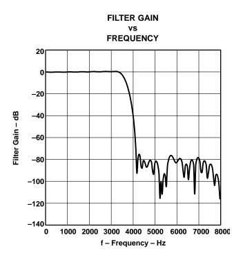
Figure 5–16. DAC FIR Frequency Response (OSR = 512)
