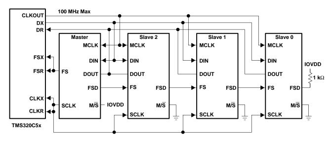
Figure 3–7. Cascade Connection (To DSP Interface)
