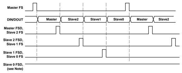
NOTE: Slave 0 FSD should be pulled high for stand-alone-master or cascade configuration. FSD must be pulled low for stand-alone-slave configuration.
