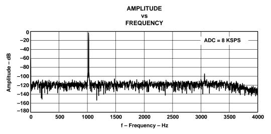
Figure 5-3. FFT—ADC Channel (-3 dB Input)
