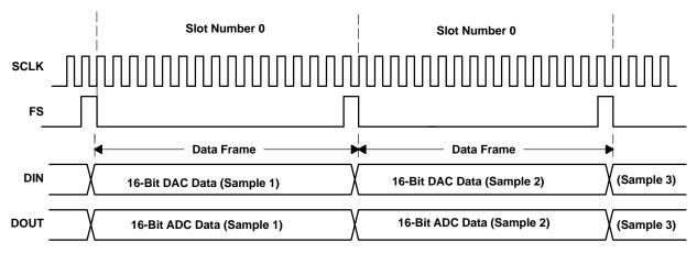
Figure 3-15. Standard Operation/Continuous Data Transfer Mode: Stand-Alone Timing
