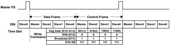
NOTE: In this example, the broadcast operation (D11 = 1) is used to program the four control registers of Reg.1, Reg.2, Reg.4, and Reg.6 in all 4 DSP codecs (Master, Slave2, Slave1, and Slave0) shown in Figure 3–8. These registers are programmed during the same frame.
