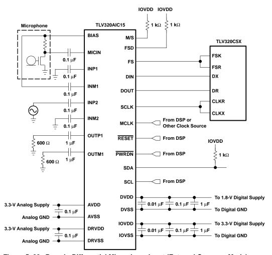
Figure 5-20. Pseudo-Differential Microphone Input (External Common Mode)
