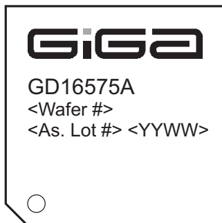
Figure 5. Device Marking, 32 pin Package - Top View
