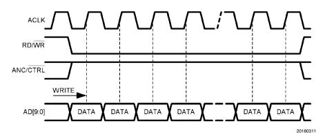
FIGURE 3. Ancillary Data Write Timing
