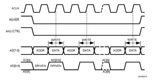
FIGURE 2. Control Data Write Timing
