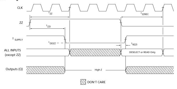
**Notes:**20. Device must be deselected when entering ZZ mode. See truth table for all possible signal conditions to deselect the device.
