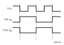
FIGURE 1. 'Worst Case Icc Test Pattern
