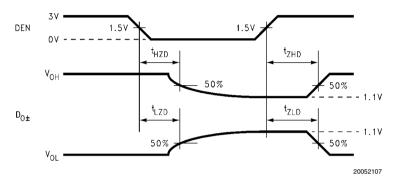
FIGURE 5. Serializer Input Clock Transition Time TRI-STATE Test Circuit and Timing
