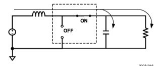
FIGURE 5. Equivalent Circuit During Cycle 2
