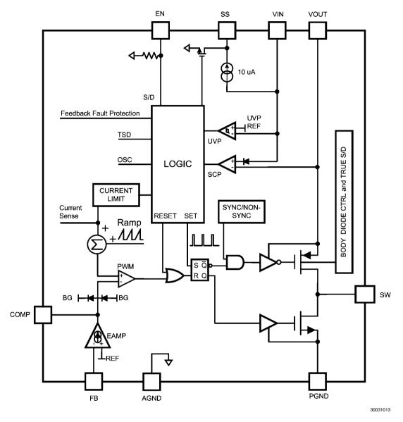
FIGURE 2. LM4510 Block Diagram
