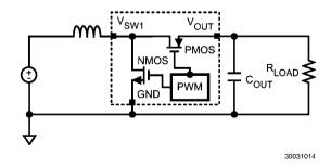
FIGURE 3. Schematic of Synchronous Boost Converter
