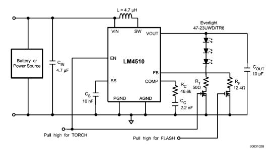
FIGURE 8. Flash/Torch Circuit Using LM4510
