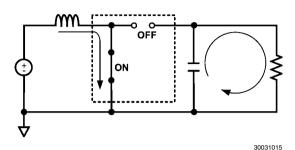
FIGURE 4. Equivalent Circuit During Cycle 1
