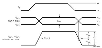
FIGURE 7. Driver Output Levels
