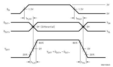
FIGURE 3. Driver Propagation Delay and Transition Time Waveforms
