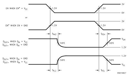
FIGURE 5. Driver TRI-STATE Delay Waveform
