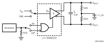
FIGURE 4. Driver TRI-STATE Delay Test Circuit
