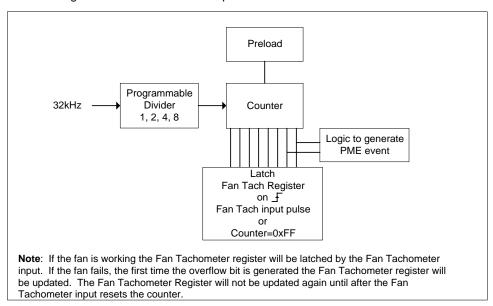
FIGURE 9 - CONCEPTUAL BLOCK DIAGRAM OF FAN MONITORING LOGIC
