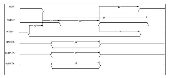
FIGURE 23 - FLOPPY DISK DRIVE TIMING (AT MODE ONLY)
