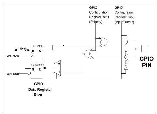
FIGURE 7 - GPIO FUNCTION ILLUSTRATION
