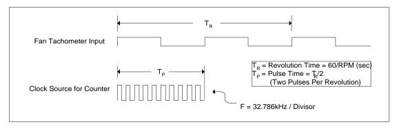
FIGURE 8 - FAN TACHOMETER INPUT AND CLOCK SOURCE
