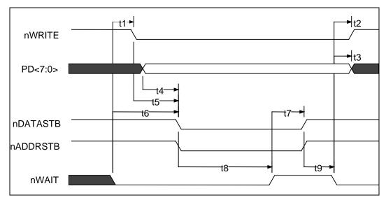
FIGURE 24 - EPP 1.9 DATA OR ADDRESS WRITE CYCLE
