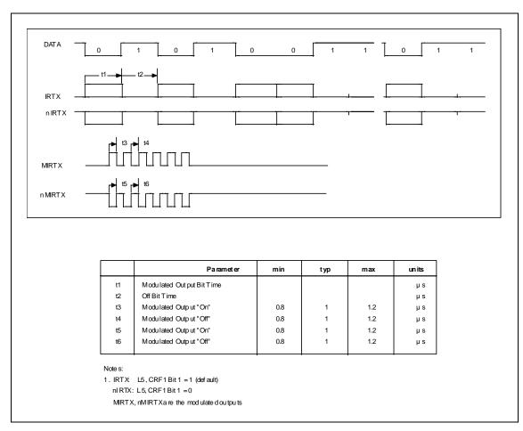
FIGURE 34 - AMPLITUDE SHIFT KEYED IR TRANSMIT TIMING
