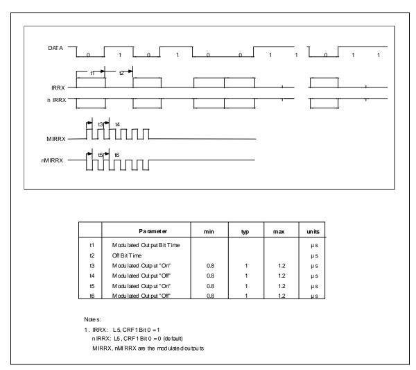
FIGURE 33 - AMPLITUDE SHIFT KEYED IR RECEIVE TIMING
