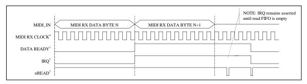
FIGURE 3 - MPU-401 INTERRUPT
