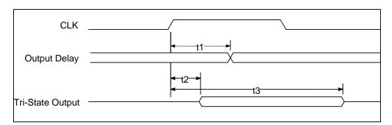
FIGURE 16 - OUPUT TIMING MEASUREMENT CONDITIONS, LPC SIGNALS
