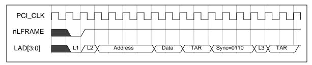
FIGURE 18 - I/O WRITE
