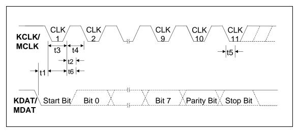
FIGURE 39 - KEYBOARD/MOUSE RECEIVE/SEND DATA TIMING
