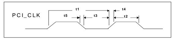
FIGURE 14 - PCI CLOCK TIMING
