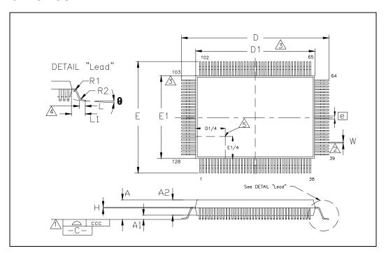
FIGURE 45 - 128 PIN QFP PACKAGE OUTLINE, 3.9MM FOOTPRINT
