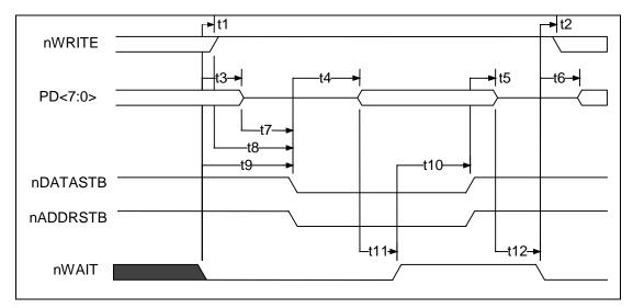
FIGURE 25 - EPP 1.9 DATA OR ADDRESS READ CYCLE
