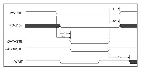
FIGURE 26 - EPP 1.7 DATA OR ADDRESS WRITE CYCLE
