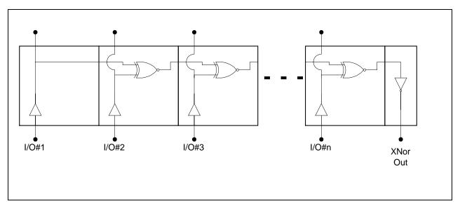
FIGURE 46 - XNOR-CHAIN TEST STRUCTURE
