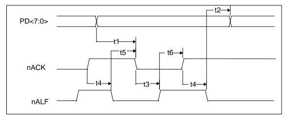
FIGURE 30 - ECP PARALLEL PORT REVERSE TIMING
