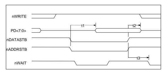
FIGURE 27 - EPP 1.7 DATA OR ADDRESS READ CYCLE
