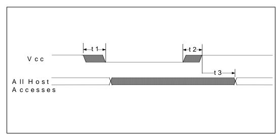
FIGURE 12 - POWER-UP TIMING
