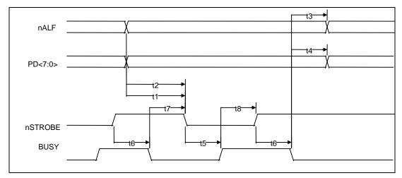
FIGURE 29 - ECP PARALLEL PORT FORWARD TIMING
