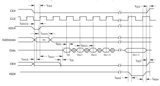
Figure 18.4 Burst Mode Read (x32 Mode)
