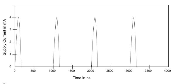
Figure 15.1  $I_{CC1}$  Current vs. Time (Showing Active and Automatic Sleep Currents)
