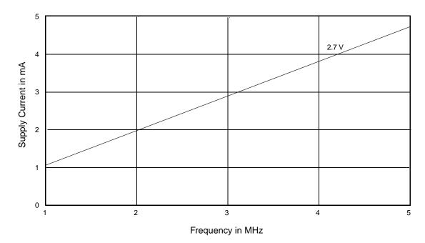
Figure 15.2 Typical I<sub>CC1</sub> vs. Frequency
