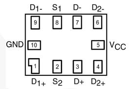
Figure 3. Micropak™ Pin Assignment (Top View)
