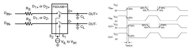
Figure 11. Skew Test
