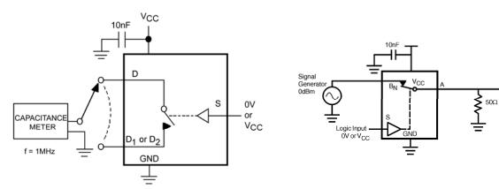
Figure 9. On/Off Capacitance Measurement Setup
