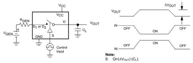
Figure 8. Charge Injection
