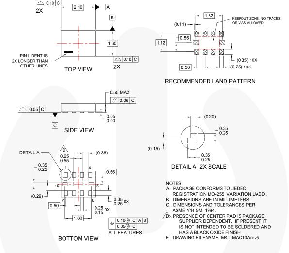
Figure 13. 10-Lead, MicroPak™, JEDEC MO255,1.6 X 2.1mm
