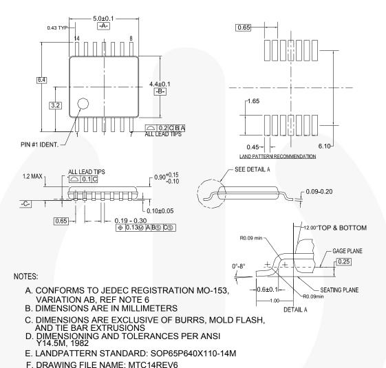
Figure 14. 14-Lead Thin Shrink Small Outline Package (TSSOP), JEDEC MO-153, 4.4mm Wide
