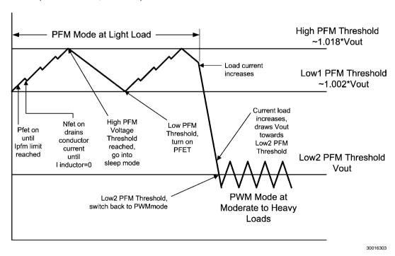
FIGURE 6. Operation in PFM Mode and Transfer to PWM Mode
