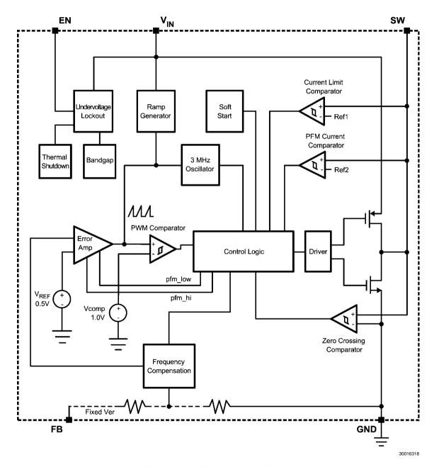
FIGURE 3. Simplified Functional Diagram
