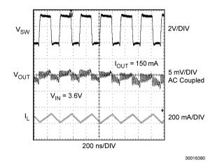
**FIGURE 4. Typical PWM Operation**
