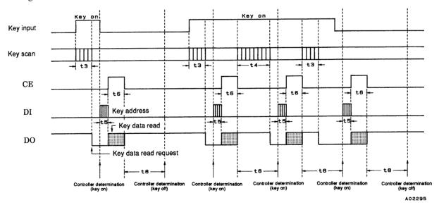
t3 ......Key scan execution time (800T [s]) when the key scan data for two key scans agrees
