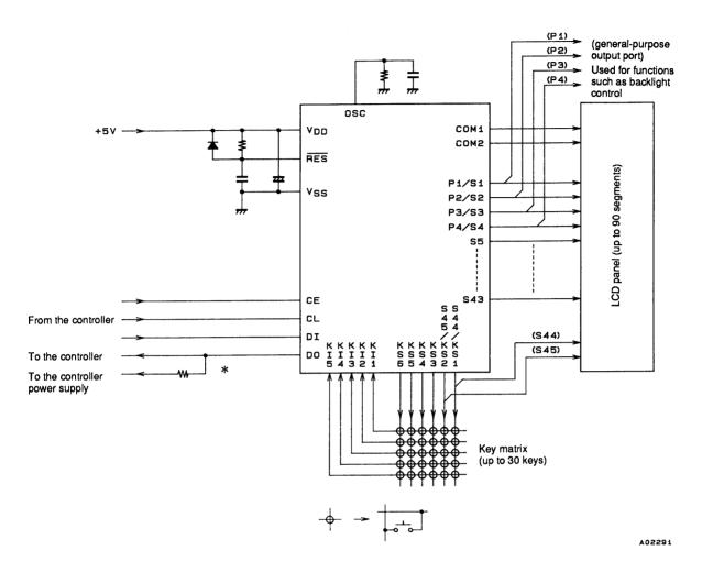
Note: \* Since DO is an open-drain output, a pull-up resistor is required. Select a value (between 1 and 10 kΩ) that is appropriate for the capacitance of the external wiring so that the waveforms are not distorted.
