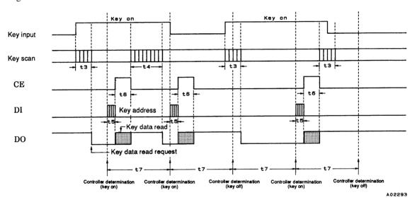
t3 ......Key scan execution time (800T [s]) when the key scan data for two key scans agrees
