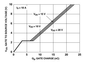
Figure 7. Gate Charge Characteristics
