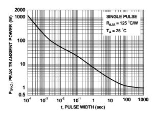
Figure 12. Single Pulse Maximum Power Dissipation
