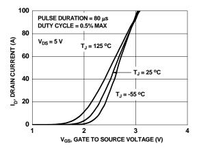
Figure 5. Transfer Characteristics
