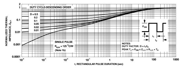
Figure 13. Junction-to-Ambient Transient Thermal Response Curve
