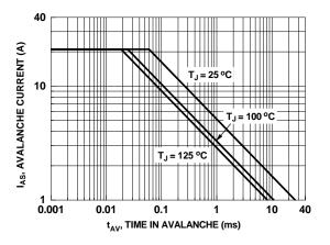
Figure 9. Unclamped Inductive Switching Capability
