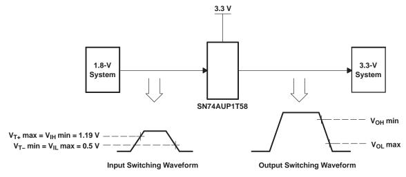
Figure 4. Switching Thresholds for 1.8-V to 3.3-V Translation
