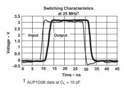
Figure 2. Excellent Signal Integrity
