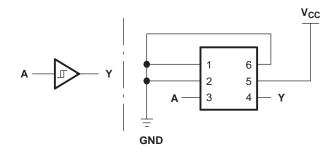
Figure 11. 17/34: Noninverted Buffer
