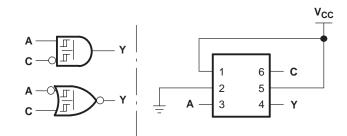
Figure 7. 14+08/14+02: 2-Input AND Gate With Inverted C Input 2-Input NOR Gate With Inverted Input
