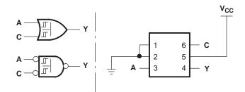
Figure 8. 32/14+00: 2-Input OR Gate 2-Input NAND Gate With Both Inputs Inverted
