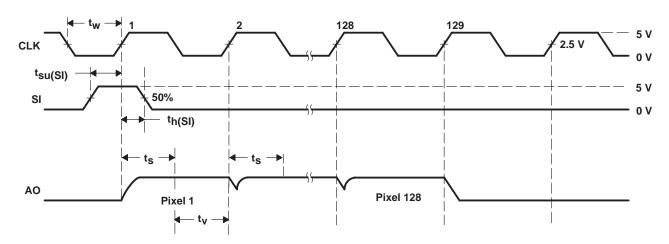
Figure 2. Operational Waveforms
