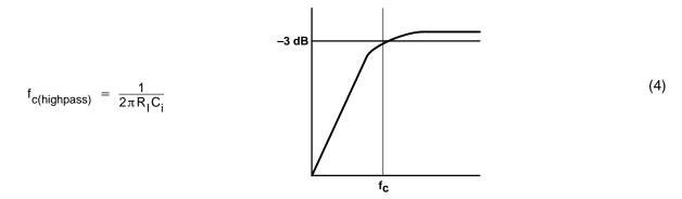
The value of C<sub>i</sub> is important to consider as it directly affects the bass (low frequency) performance of the circuit. Consider the example where R<sub>I</sub> is 710 k $\Omega$  and the specification calls for a flat bass response down to 40 Hz. Equation 2 is reconfigured as equation 5.
