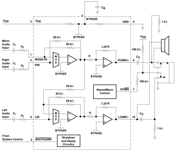
Figure 25. TPA0223 Resistor Divider Network Circuit
