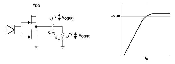
Figure 23. Single-Ended Configuration and Frequency Response
