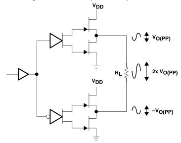
Figure 22. Bridge-Tied Load Configuration
