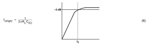
The main disadvantage, from a performance standpoint, is that the load impedances are typically small, which drives the low-frequency corner higher, degrading the bass response. Large values of C(C) are required to pass low frequencies into the load. Consider the example where a C(C) of 330 µF is chosen and loads vary from 3  $\Omega$ , 4  $\Omega$ , 8  $\Omega$ , 32  $\Omega$ , 10 k $\Omega$ , to 47 k $\Omega$ . Table 1 summarizes the frequency response characteristics of each configuration.
