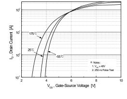
Figure 2. Transfer Characteristics
