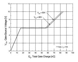
Figure 6. Gate Charge Characteristics
