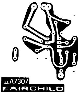
Fig. 3 1:1 Scale P.C. Board Layout for Circuit of Figure 1
