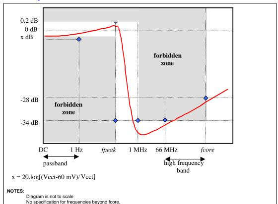
Figure 29. PLL Filter Specifications
