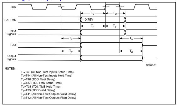
**Figure 16. Test Reset Timings**
