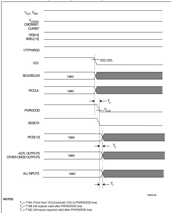
Figure 13. Power Down Sequencing and Timings (VCC Leading)
