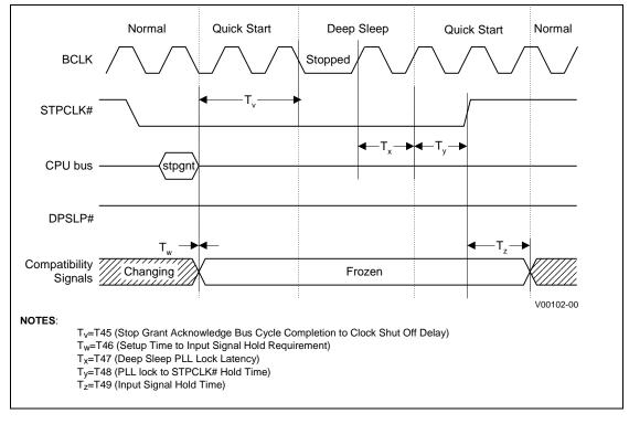
Figure 17.Quick Start/Deep Sleep Timing (BCLK Stopping Method)
