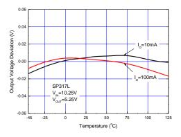
Figure 4. Load Regulation vs. Temperature
