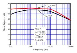
Figure 11. Ripple Rejection vs. Frequency
