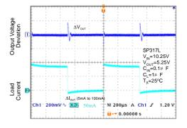
Figure 12. Load Transient Response
