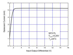
Figure 9. Minimum Operating Current
