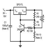
Figure 15. 5V Logic Regulator with Electronic Shutdown (Minimum output = 1.2V)
