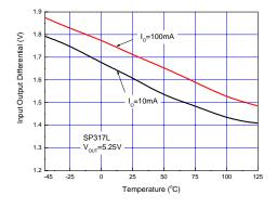
Figure 8. Dropout Voltage vs. Temperature
