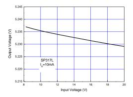
Figure 5. Output Voltage vs. Input Voltage
