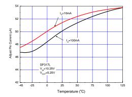
Figure 7. Adjustment Current vs. Temperature
