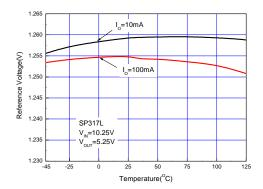
Figure 6. Reference Voltage vs. Temperature
