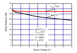
Figure 10. Ripple Rejection vs. Output Voltage
