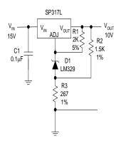
Figure 17. High Stability 10V Regulator
