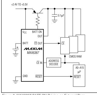
Figure 3. MAX6367 BATT ON Driving an External Pass Transistor
