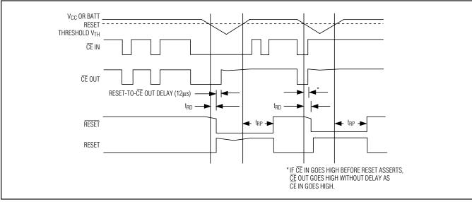
Figure 1. Reset and Chip-Enable Timing
