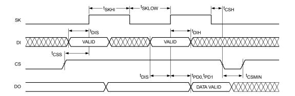
Figure 1. Sychronous Data Timing
