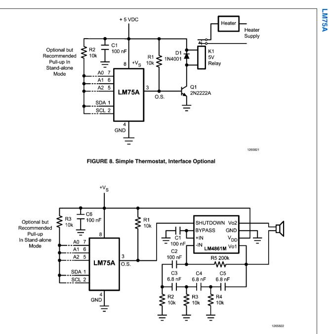
FIGURE 9. Temperature Sensor with Loudmouth Alarm (Barking Watchdog)
