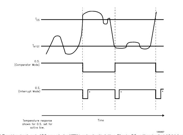
Note 15: These interrupt mode resets of O.S. occur only when LM75A is read or placed in shutdown. Otherwise, O.S. would remain active indefinitely for any event.
