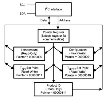
There are four data registers in the LM75A and an additional Product ID register selected by the Pointer register. At powerup the Pointer is set to "000"; the location for the Temperature Register. The Pointer register latches whatever the last location it was set to. In Interrupt Mode, a read from the LM75A, or placing the device in shutdown mode, resets the O.S. output. All registers are read and write, except the Temperature register and the LM75A's Product ID register, which are read only.
