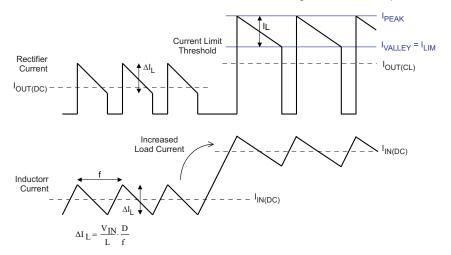
Figure 21. Inductor/Rectifier Currents in Current Limit Operation
