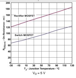
Figure 19. MOSFET r<sub>DS(on)</sub> vs Temperature
