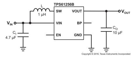
Figure 20. Parameter Measurement Schematic
