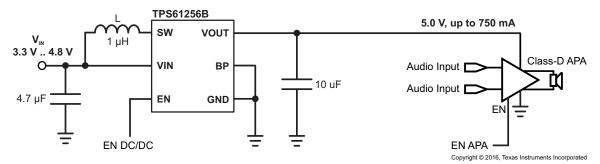
Figure 33. "Boosted" Audio Power Supply
