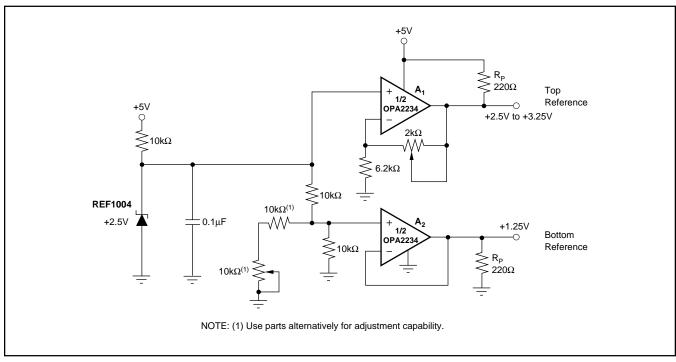
FIGURE 11. Optional External Reference to Set the Full-Scale Range Utilizing a Dual, Single-Supply Op Amp.
