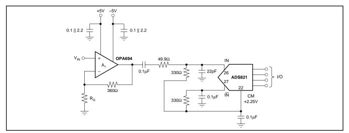
FIGURE 6. Low-Cost, AC-Coupled, Single-Ended Input Circuit.
