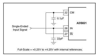
FIGURE 10. Single-Ended Input Connection.
