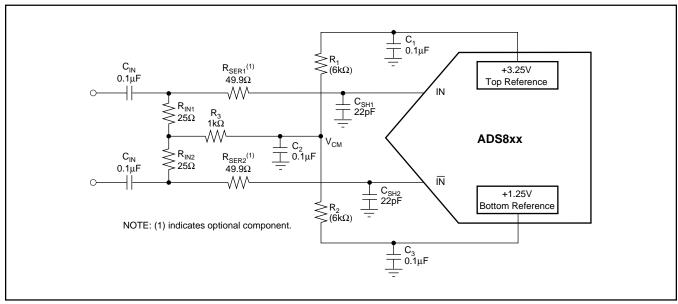
FIGURE 7. AC-Coupled Differential Input Circuit.
