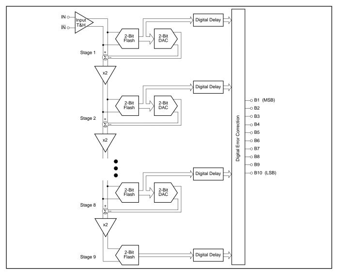
FIGURE 2. Pipeline A/D Converter Architecture.
