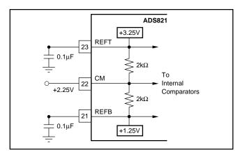
FIGURE 3. Internal Reference Structure.
