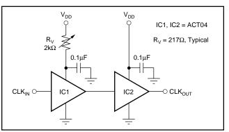
FIGURE 4. Clock Skew Circuit.
