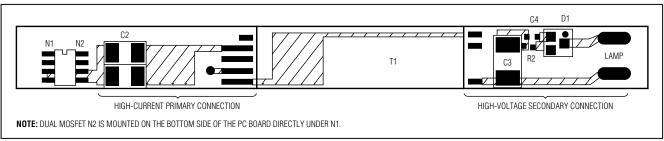
Figure 10. High-Voltage Components Layout Example
