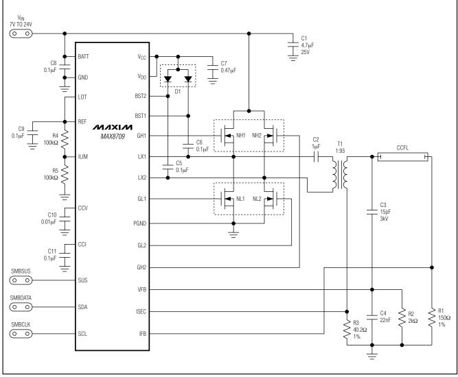
Figure 1. Typical Operating Circuit of the MAX8709
