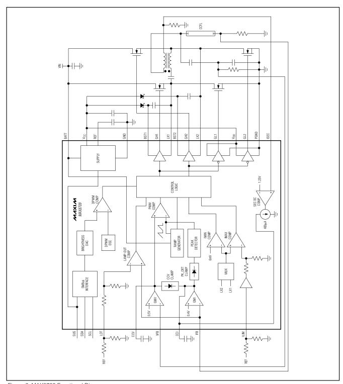
Figure 2. MAX8709 Functional Diagram
