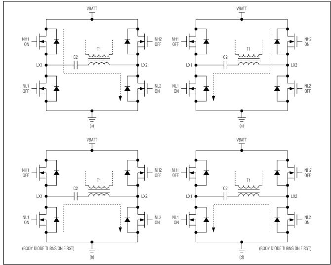
Figure 3. Resonant Operation
