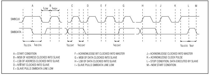
Figure 8. SMBus Write Timing
