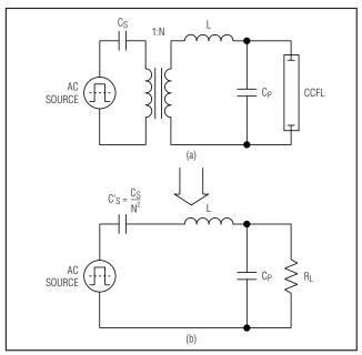
Figure 4. Equivalent Resonant Tank Circuit
