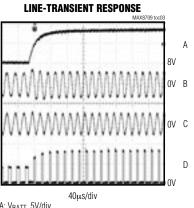
A: V<sub>BATT</sub>, 5V/div B: V<sub>IFB</sub>, 2V/div C: V<sub>VFB</sub>, 2V/div D: V<sub>LX1</sub>, 10V/div
