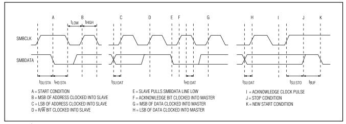
Figure 9. SMBus Read Timing
