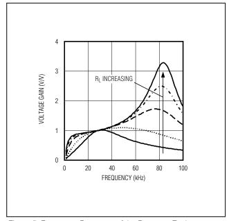
Figure 5. Frequency Response of the Resonant Tank
