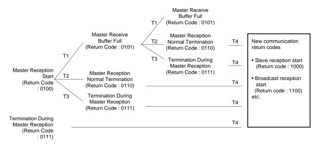
The minimum generation intervals for return codes in master transmission are shown below.
