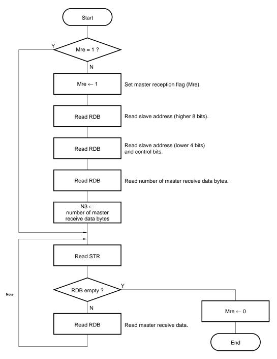
Note To distinguish data from receive data (slave reception, broadcast reception) newly input in the next communication frame, after reading RDB (inputting one serial clock pulse to  $\overline{SCK}$  pin), STR should be read (inputting one serial clock pulse to  $\overline{SCK}$  pin) within the time shown below.
