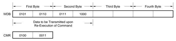
The previously set MREQ1 command values are used for the broadcast bits, control bits and number of transmit data bytes.
