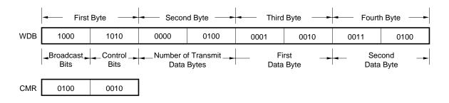
Caution Transmit data 56H and 78H should be set when the above command parameters have been read and WDB is empty.
