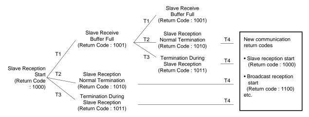
The minimum generation intervals for return codes in master transmission are shown below.
