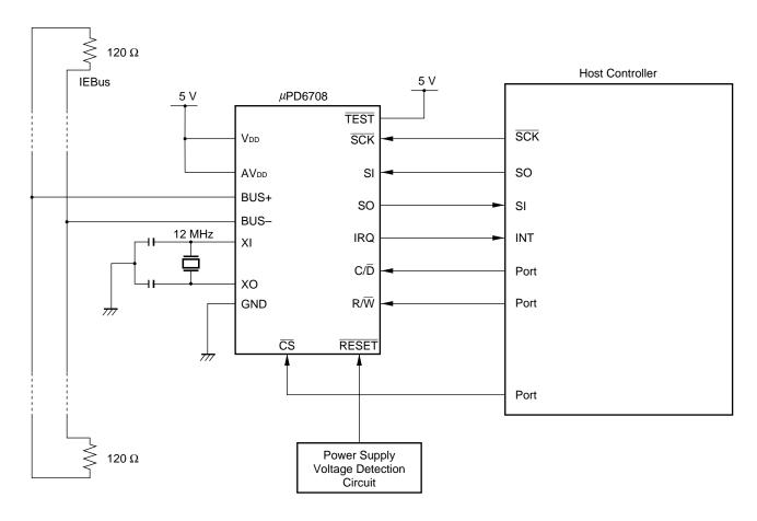
Caution If the power supply voltage moves out of the 5 V  $\pm$ 5 % range, the  $\overline{\text{RESET}}$  pin must be driven low for 6  $\mu$ s or more in order to reset the  $\mu$ PD6708.
