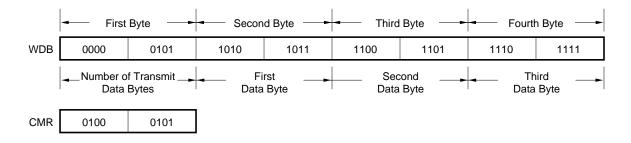
Caution Transmit data 14H and 25H should be set when the above command parameters have been read and WDB is empty.
