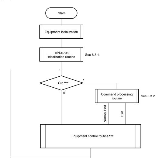
**Note** The equipment control routine is a routine which performs host controller application processing. When controlling the  $\mu$ PD6708, set the Crq flag when there is a command request.
