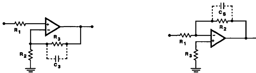
FIGURE 21. SUGGESTED STABILITY CIRCUITS
