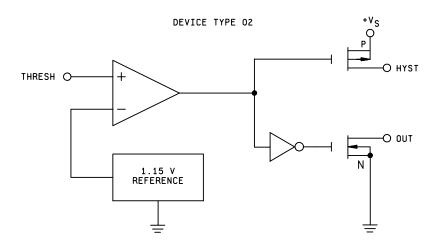
FIGURE 2. Block diagram.
