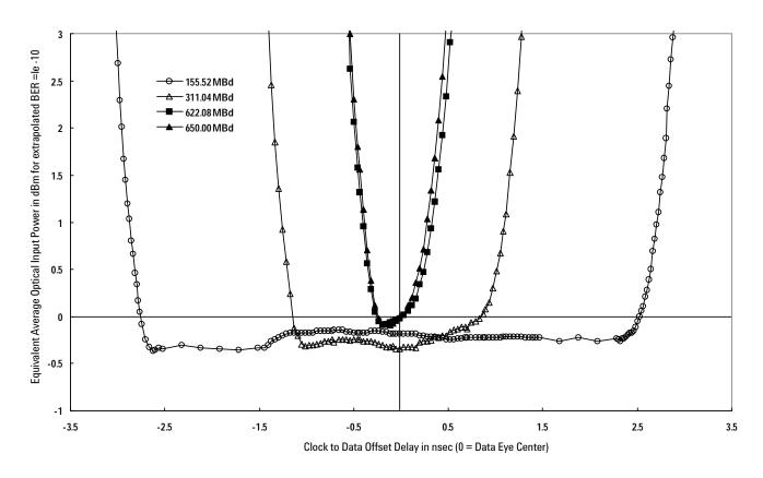
Figure 2. HFBR-5208xxMZ Relative Input Optical Power as a function of sampling time position. Normalized to center of Baud interval at 622 MBd. Test Conditions +25°C, 5.25 V, PRBS  $2^{23}$ -1, optical  $\tau_r/\tau_f=0.9$  ns with 3 m of 62.5  $\mu$ m MMF.
