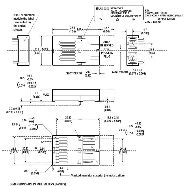
Note 1: HFBR-5208xxxZ uses LED transmitter and therefore "ZZZZ LASER PROD" will not be printed on the label.
