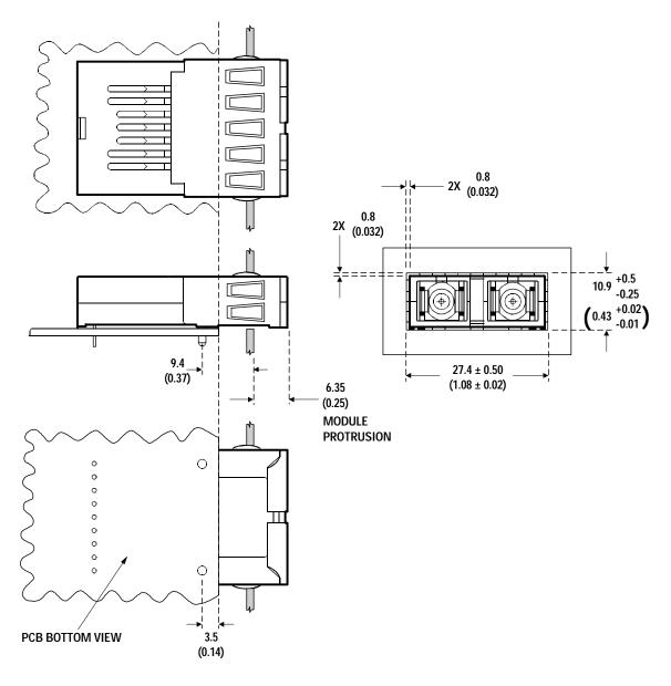
DIMENSIONS ARE IN MILLIMETERS (INCHES). TOLERANCES: X.XX  $\pm 0.025 \ \text{mm} \\ \text{X.X} \pm 0.05 \ \text{mm}$  UNLESS OTHERWISE SPECIFIED.
