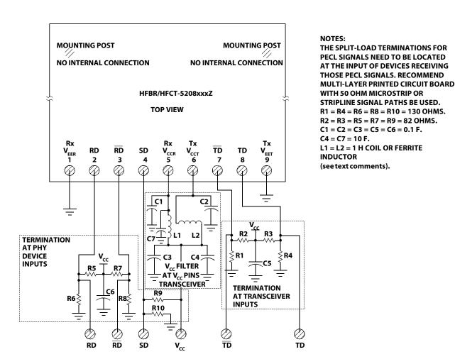
Figure 4. Recommended Circuit Schematic for dc Coupling (at +5 V) between Optical Transceiver and Physical Layer IC
