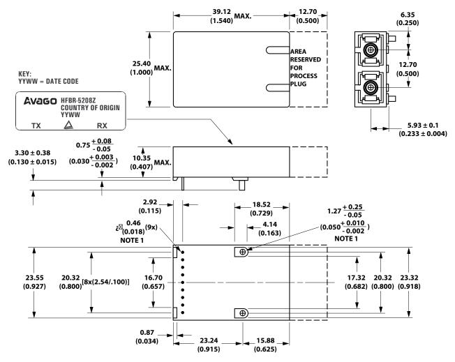
NOTE 1: PHOSPHOR BRONZE IS THE BASE MATERIAL FOR THE POSTS & PINS. FOR LEAD-FREE SOLDERING, THE SOLDER POSTS HAVE TIN COPPER OVER NICKEL PLATING, AND THE ELECTRICAL PINS HAVE PURE TIN OVER NICKEL PLATING.
