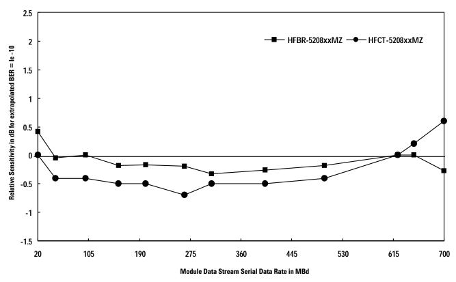
Figure 3. Relative Input Optical Power as a function of data rate normalized to center of Baud interval at 622 MBd. Test Conditions  $+25^{\circ}$ C, 5.25 V, PRBS  $2^{23}$ -1, optical  $\tau_r/\tau_f=0.9$  ns with 3 m of MMF or SMF.
