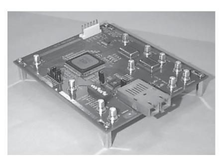
Figure 6. 622.08 Mb/s OC-12 ATM-SONET/SDH Reference Design Board
