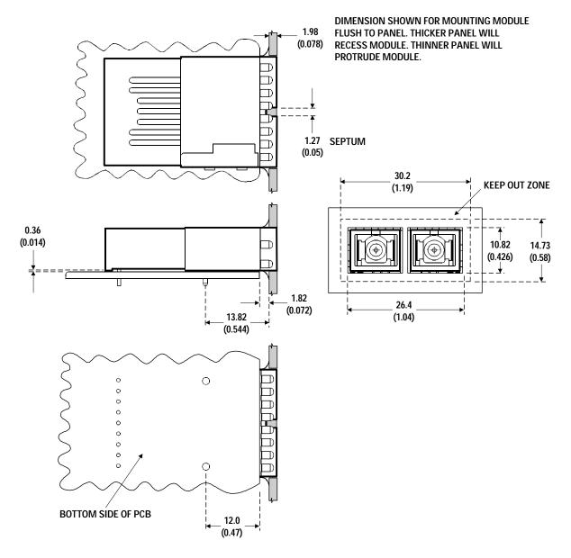
DIMENSIONS ARE IN MILLIMETERS (INCHES). TOLERANCES: X.XX  $\pm 0.025 \ mm$  UNLESS OTHERWISE SPECIFIED.
