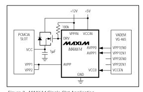
Figure 2. MAX614 Single-Slot Application
