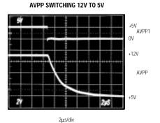
$C_{VPPIN} = 1\mu F$ ,  $AVPP0 = \overline{AVPP}1$ ,  $C_{AVPP} = 0.1\mu F$
