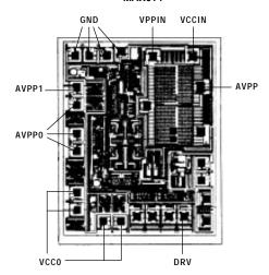
TRANSISTOR COUNT: 982; SUBSTRATE CONNECTED TO GND.
