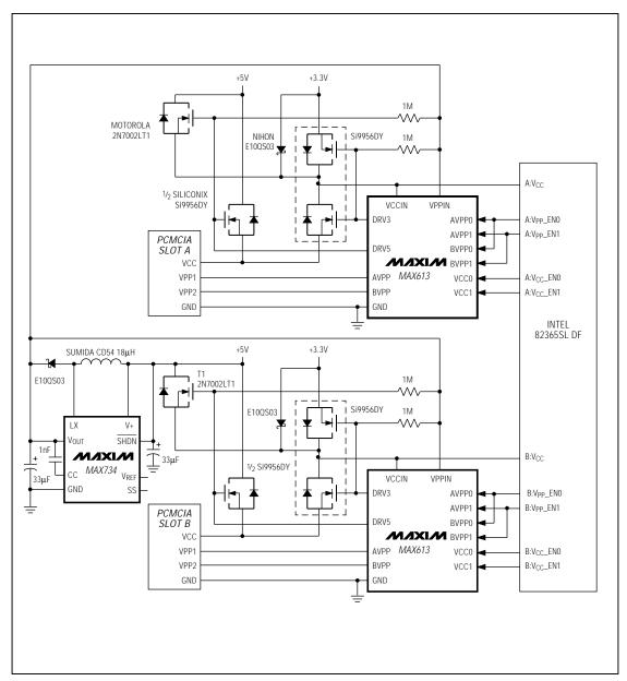
Figure 4. Mixed 3.3V/5V VCC Application Circuit
