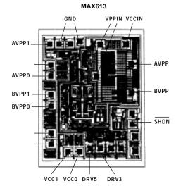
TRANSISTOR COUNT: 982; SUBSTRATE CONNECTED TO GND.
