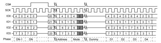
Figure 10.27 Quad I/O Read Command Sequence (4-Byte Address, ECh or EBh [CR2V[7]=1])
