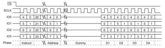
Figure 10.17 Read Any Register, QPI Mode, CR2[7] = 1 Command Sequence
