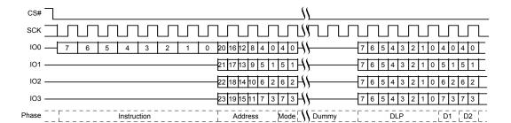
Figure 10.30 DDR Quad I/O Read Initial Access (3-Byte Address, EDh [CR2V[7]=0)
