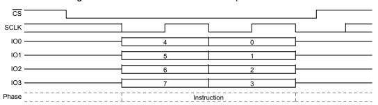
Figure 10.63 Software Reset Command Sequence QPI Mode
