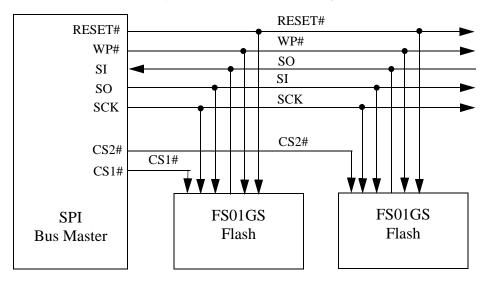
Figure 3.2 Bus Master and Memory Devices on the SPI Bus - Dual Bit Data Path
