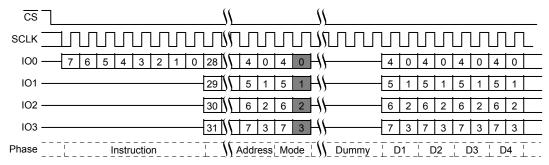
Figure 4.10 Quad I/O Read Command in QPI Mode
