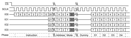
Figure 10.24 Quad I/O Read Command Sequence (3-Byte Address, EBh [CR2V[7]=0])
