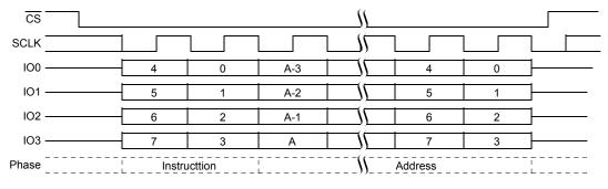
Figure 10.42 Bulk Erase Addressed Command Sequence QPI Mode
