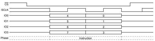
Figure 10.65 Mode Bit Reset Command Sequence QPI Mode
