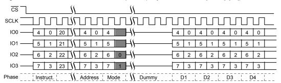
Figure 10.26 Continuous Quad I/O Read Command Sequence (3-Byte Address)
