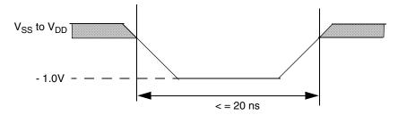
Figure 5.2 Maximum Positive Overshoot Waveform
