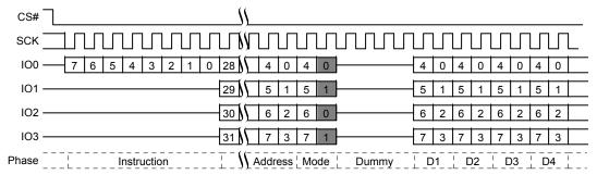
Figure 10.28 Continuous Quad I/O Read Command Sequence (4-Byte Address)
