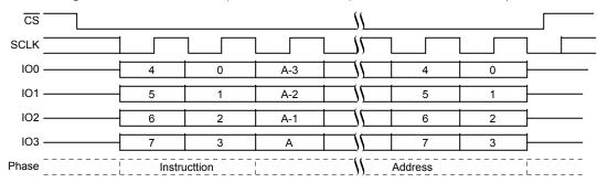
Figure 10.40 Sector Erase (SE D8h or 4SE DCh) QPI Mode Command Sequence
