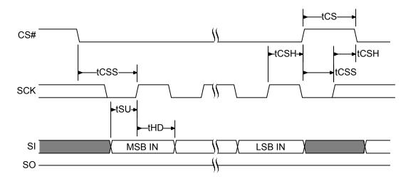
Figure 6.11 SPI Single Bit Output Timing
