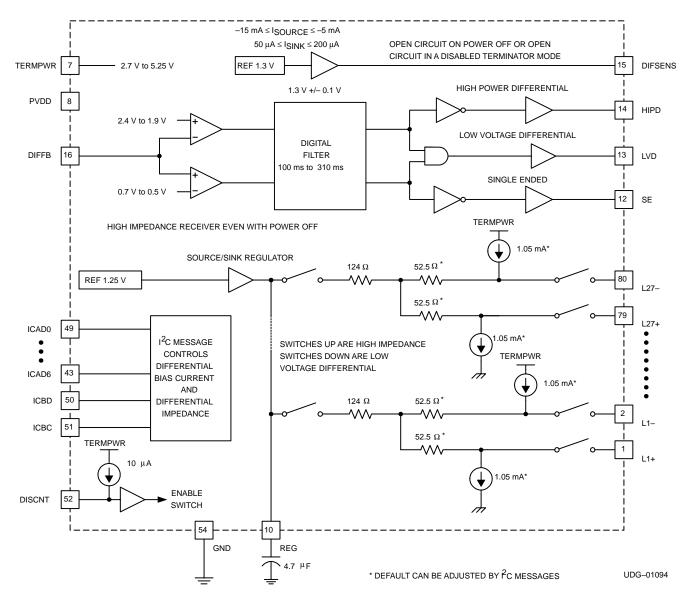
The DIFF SENSE line is driven by the terminator and monitored by the terminator DIFF B input pin. DIFF B has a digital filter and a 100-ms to 310-ms delay before the mode of the terminator is changed to reflect the new DIFF B input level. A set of comparators that allow for ground shifts determines the bus status as follows: any DIFF SENSE signal below 0.5 V is single ended, between 0.7 V and 1.9 V is LVD SCSI, and above 2.4 V is HVD SCSI.
