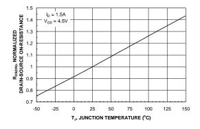
Figure 3. On-Resistance Variation withTemperature.
