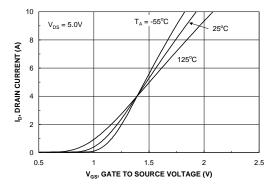
Figure 5. Transfer Characteristics.
