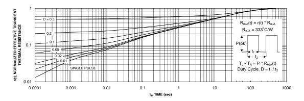
Figure 11. Transient Thermal Response Curve.
