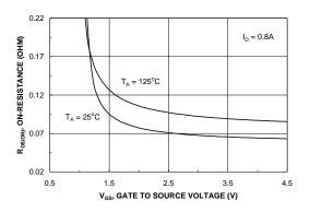
Figure 4. On-Resistance Variation with Gate-to-Source Voltage.
