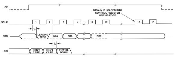
Figure 3. Serial Interface Diagram
