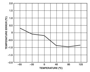
Figure 6. Typical Temperature Error @ 2.65 V
