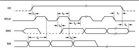
Figure 1. Timing Diagram
