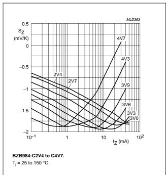
Temperature coefficient as a function of working current; typical values.
