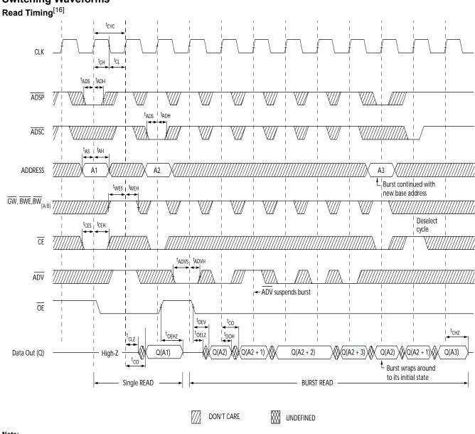
Note: 16. On this diagram, when  $\overline{CE}$  is LOW,  $\overline{CE}_1$  is LOW,  $\overline{CE}_2$  is HIGH and  $\overline{CE}_3$  is LOW. When  $\overline{CE}$  is HIGH,  $\overline{CE}_1$  is HIGH or  $\overline{CE}_2$  is LOW or  $\overline{CE}_3$  is HIGH.
