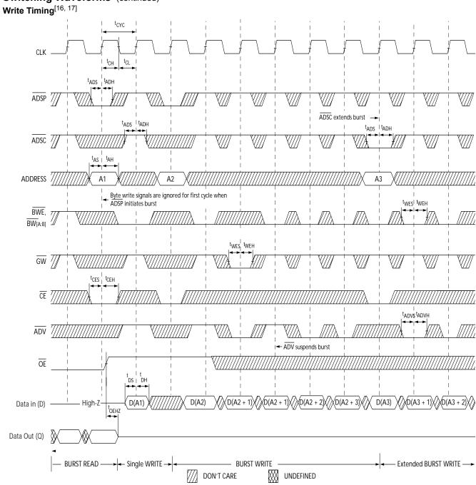
**Note:** 17. Full width write can be initiated by either  $\overline{\text{GW}}$  LOW; or by  $\overline{\text{GW}}$  HIGH,  $\overline{\text{BWE}}$  LOW and  $\overline{\text{BW}}_{[A:B]}$  LOW.
