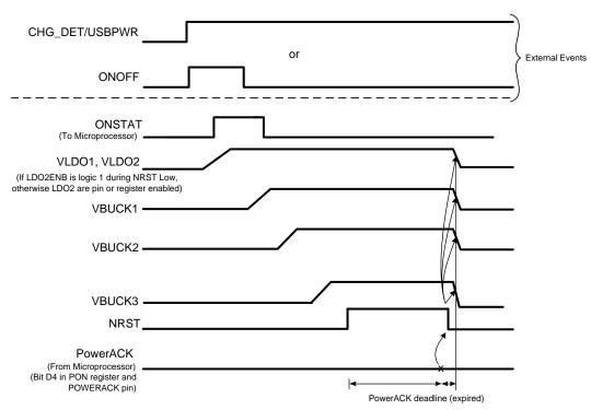
Power Down Caused by Expiring PowerACK deadline
