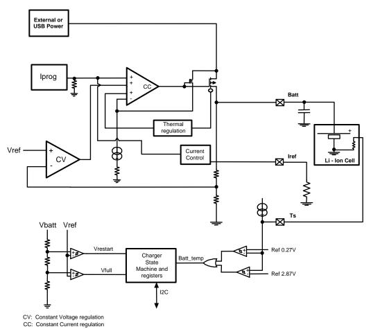
The charger module is a linear charger with constant current pre-qualification, constant current ("CC") full-rate charging and constant voltage ("CV") charging. CC and CV regulation is performed using an internal Power FET Q2 with reverse current blocking. The termination voltage is controlled to within ±0.35% at room temperature.
