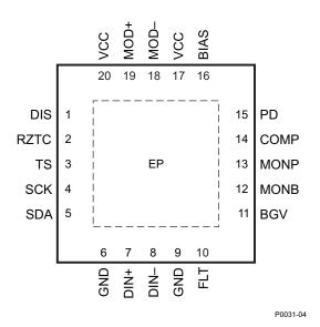
Figure 4. Pinout of ONET1191V in a 4-mm  $\times$  4-mm, 20-Pin QFN Package
