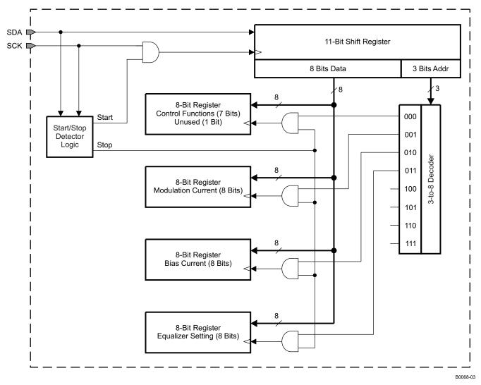
Figure 2. Simplified Two-Wire Interface Block Diagram
