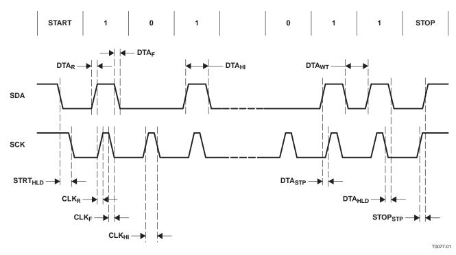
Figure 3. Two-Wire Interface Timing Diagram
