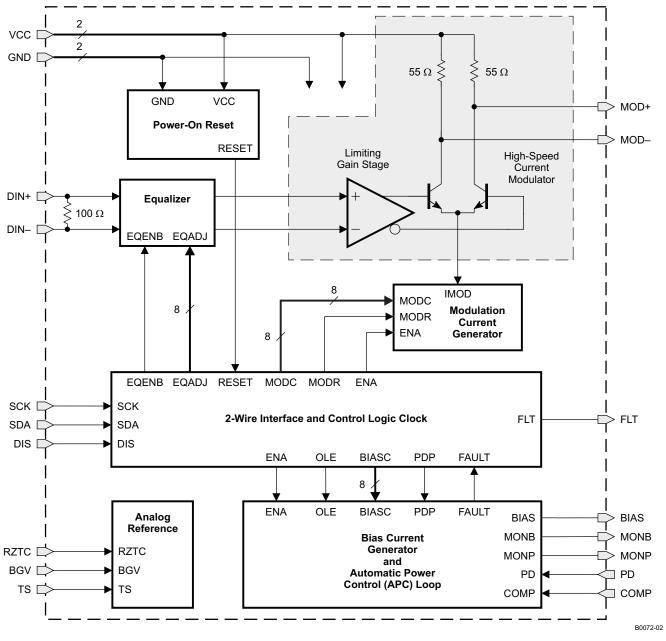
Figure 1. Simplified Block Diagram of the ONET1191V
